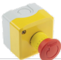
AC65529 Emergency push-button 2 NC 3A - EN ISO 13850 It must interrupt the power supply line of the gate in case of emergency - PG 13.5 cable passage hole (Ø12) - IP 66 - 68x68x92.5 mm
